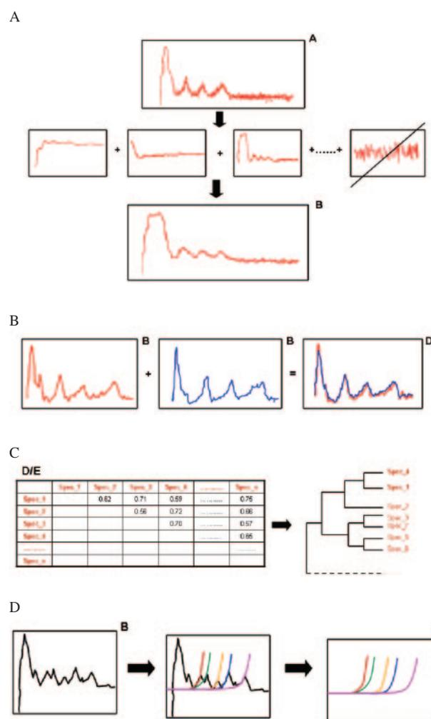
**Fig. 2.** Algorithm for noise reduction, alignment and clustering of force curves. (A) Noise reduction: Dimension reduction with singular value decomposition is applied. (B) Curve alignment: The two curves are aligned with dynamic programming. (C) Clustering: The pairwise distances obtained with curve alignment are clustered with hierarchical clustering and average linkage. (D) Peak detection: Peaks are detected with the worm-like chain model for evaluation of the clustering.
